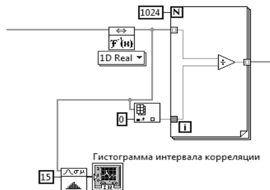
Figure 11 – A fragment of the program code responsible for performing an inverse fast Fourier transform and performing normalization of the ACF.
