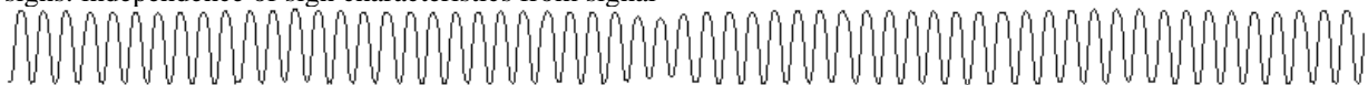
Figure 1 – A fragment of the signal reflected from the car traveling at a speed of 30-40 km/h, the duration of the fragment is 100 ms.
